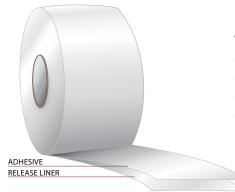
**Transfer tapes** or unsupported tapes have a coating of adhesive on one side of a double sided release liner. There is no additional backing or supporting material. These tapes can be converted into other types of tape product by lamination to another material, or can be used directly to bond two materials together.
