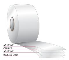
**Double coated tapes** have an adhesive coated on both sides of a central carrier, often a thin (0.5 mil) polyester, but many films, papers, foams and more can be used. These products also use release liner, which is normally also double sided and uses a differential release to enable easy unwind and application. The adhesive on each side of the carrier can be the same, or different. Similarly, the two adhesives can be the same or different thicknesses.
